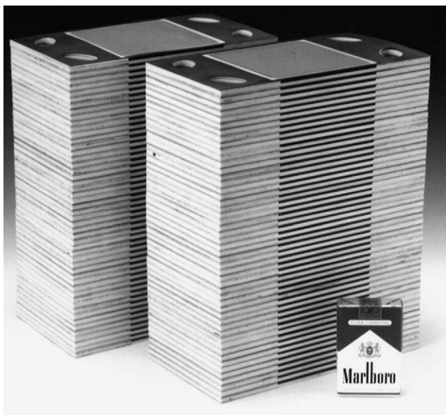
Fig. 2. Photograph of a pair of 48-cell stacks for an electrolyte-supported type SOFC.
